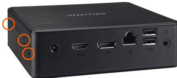
WLAN antenna perforations and Kensington Lock hole
